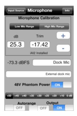
To begin calibration, select Low Range (darker). Select gain range +10 as a starting point (see picture below). Turn on Phantom Power, if required by your microphone. Now attach and turn on your calibrator. Leave the calibrator running for the remainder of this procedure.
